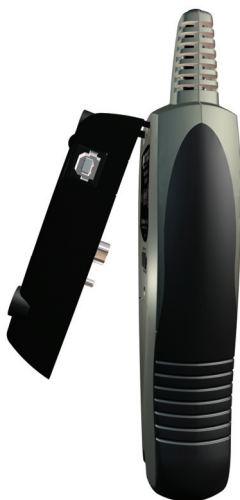
Figure 5-1 Connecting the Dock
