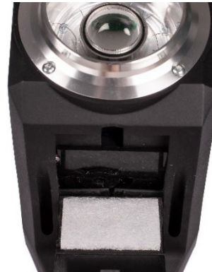
Figure 65: Inlet filter replacement
