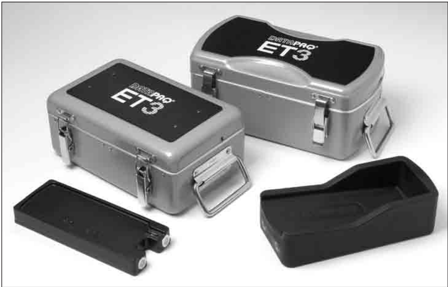
EasyTrack3 aluminum thermal barriers and their heatsinks: TB0253 (left) and TB0263 (right).
