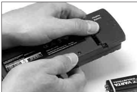
Opening the battery-compartment door.
