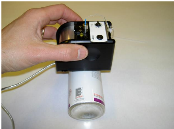
Fig. 5.1 Testing curved surfaces perpendicular to the object axis
