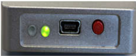
Flashing Green LED: Active Data Collection
