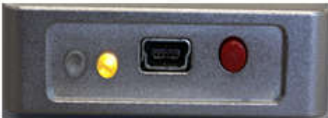
Flashing Yellow LED: Unit in Pause
