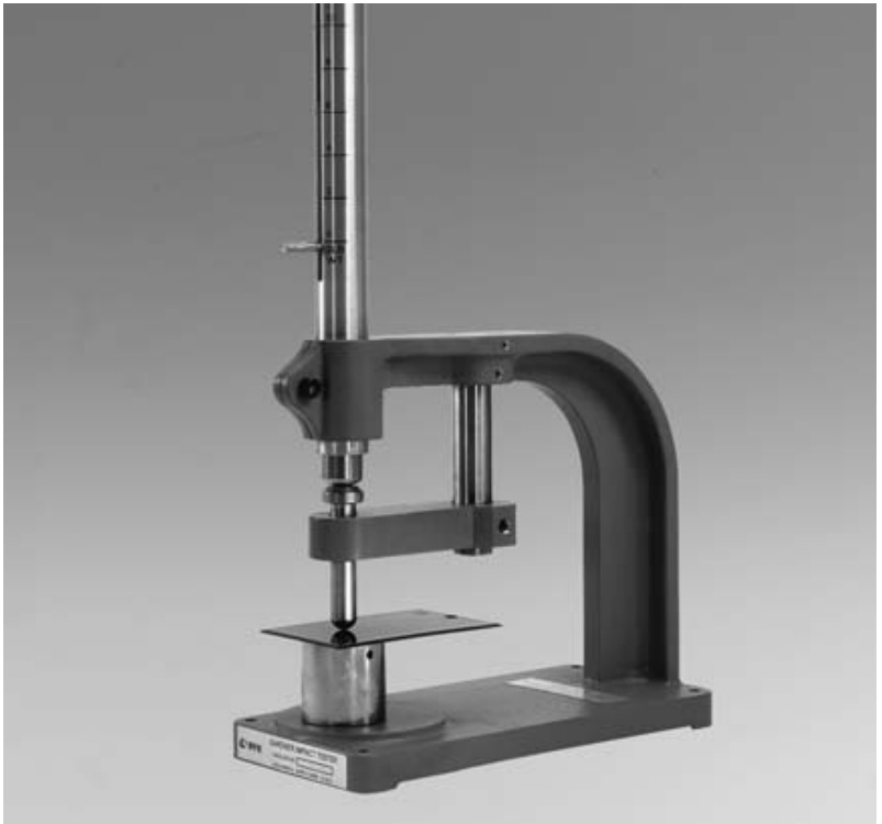
Illustration 1: BYK-Gardner Heavy-Duty Variable Height Impact Tester
