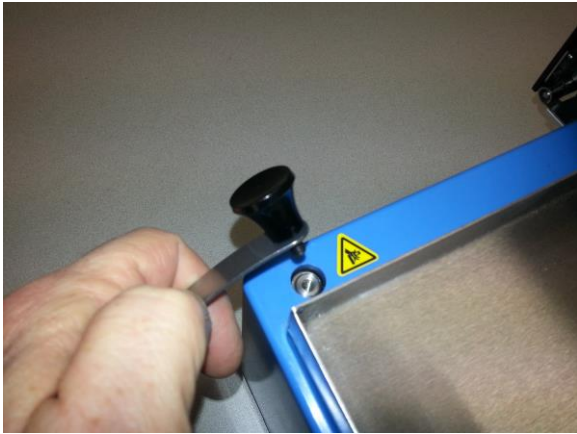
Push the knob into the spring
