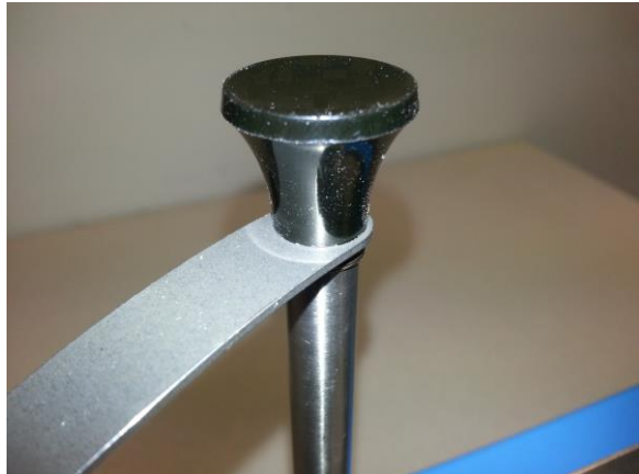
Grasp the shaft and tighten the knob fully
