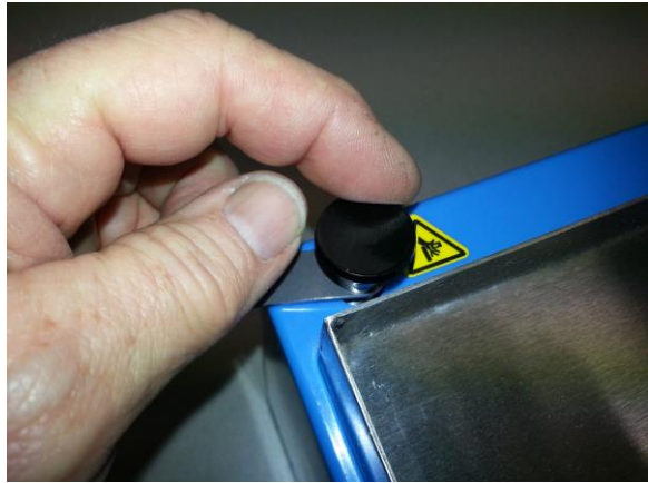
Screw the knob into the shaft
